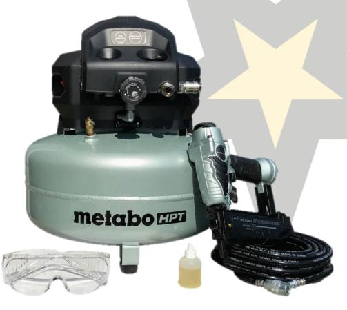
THE KNT50ACM FINISH COMBO KIT FROM METABO HPT IS IDEAL FOR A WIDE VARIETY OF FINISH WORK AND CABINETRY PROJECTS. IT COMES COMPLETE WITH A 6-GALLON PANCAKE COMPRESSOR THAT FEATURES AN OIL-FREE HIGH EFFICIENCY 1-HP MOTOR, CAPABLE OF PRODUCING 2.8 CFM AT 90 PSI, AND THE NT50AE2 2" 18-GAUGE BRAD NAILER, WHICH IS IDEAL FOR TRIM WORK, FURNITURE BUILDING AND OTHER FINISH APPLICATIONS. ALSO INCLUDES A 25 FT. HYBRID HOSE, SAFETY GLASSES AND PNEUMATIC OIL.
