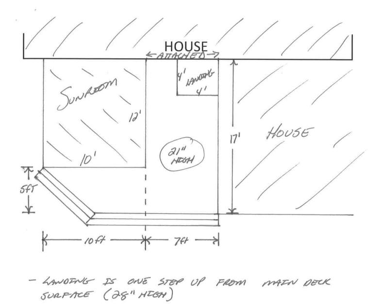
Make sure to have ALL measurements noted on drawing. Include location and width of the stairs.
